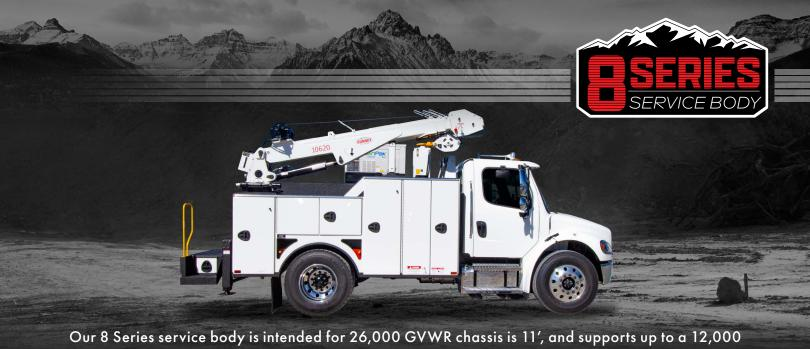
Our 8 Series service body is intended for 26,000 GVWR chassis is 11', and supports up to a 12,000 lbs. capacity crane. They're built for strength and durability and will perform in rough conditions for years to come. The body has abundant storage for tools and accessories to ensure field service techs arrive at the job site prepared to complete any task.
