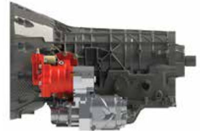
DTM 70 CFM PTO driven, direct transmission mounted, air compressor
